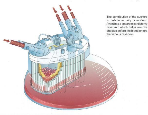
In an open system the risk of emboli to the patient due to a low level within the reservoir is often reduced by a low level detector. When, however, this system is not available or fails, Sorin Group patented safety valve comes to your help.
